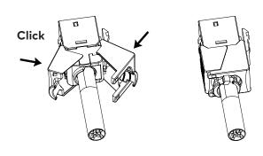
If you don't have the copper tape please connect the drain wire to the shielded Shell housing and tie up the cable tie.
