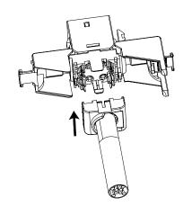
Close the outer cap by pushing down both sides until it clicks. For more security please tie up the cable tie that is in the packaging.
