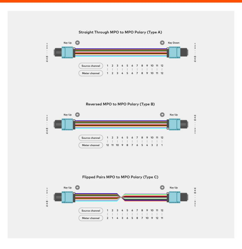
MPO/MTP have several benefits compared to other connectors, including the fact that they are quick to install, they don't need to be merged and they don't take up much space, it's possible to have a connector with 12 fibers, for example, instead of having 12 individual connectors. In this aspect, they prove to be a
