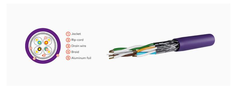
Cable Cat.6A S/FTP LSZH CU 4P AWG23 barpa construction
