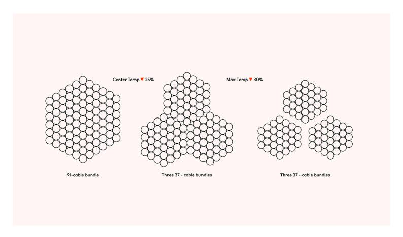
Impact of cable number reduction and separation (assuming Cat. 6A, 1000mA 4-pair cables)
