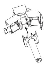
Close the outer cap by pushing down both sides until it clicks. For more security please tie up the cable tie that is in the packaging.
