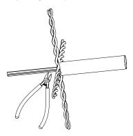
Insert the pairs throught the cap slots according to TIA568A/B wiring instruction label and trim the wires flush.
