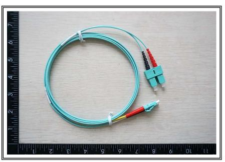
Test item: Fiber Patch Cord Tested Model: 812T2AACCMM (T refer to category, AA refer to first connector and MM refer to meters)
