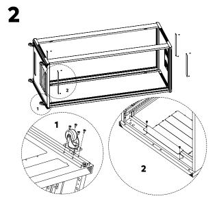
With the cable entry panel (9) and with the castors (10), assemble in the bottom plate with  $24 \times bolt M5*10$  (A);
