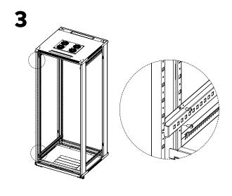
With the cabinet in the vertical, assemble the mounting angle **(4)** with  $16 \times 12$  **(B)** in the horizontal sides of the cabinet;
