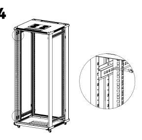
Grab the 19" rails (3) in the vertical and mount with 16 x bolt M6\*12 (B);
