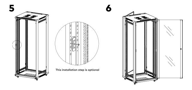
This installation step is optional. With  $2 \times bolt M5*10$  (A) fix this accessory to the frame;
