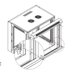
Install front frame by 4pcs of M6\*12 screws (6pcs of M6\*12 screws if more than 18U), refer to the picture;
