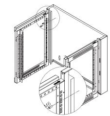
Install side frames to the grooves of back frame by 4pcs of M6\*12 screws (6pcs if more than 18U) as shown by the arrow in the picture, note 19" mounting rails are in the front side;
