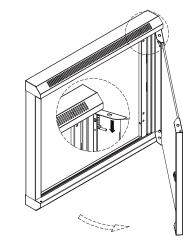
Open the front door by key, pull the door latch downward, refer to the picture, remove the front door from front frame, put them separate for the preparation of the frame assembly;
