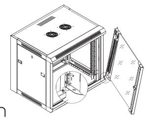
Repetition step 2, install front door. Tip: SE enclosure is the bolted structure, need to adjust the diagonal size of enclosure after the assembly, ensure homogeneous space for all doors and doors work well.
