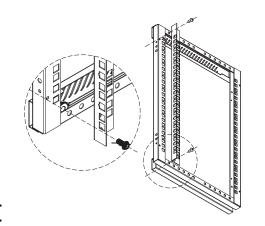
Fix 19" mounting rails to the first holes of top & bottom of side frames by 4sets of M5 screws;
